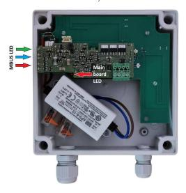
On the side of the device are five MBUS LEDs which indicate according to the table below.
