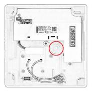
5. Take the device and hold it where it is going to be mounted. Mark the holes, pre-drill if necessary (depending on the material), and mount the device by using four screws (not included).
