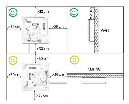
Find a suitable place to install the repeater. If indoors, then walls are recommended. If outdoors, then walls, poles, or similar works great. To mount a repeater on poles, it's recommended to use the Lansen pole mounting kit (article number LAN-910-0066).
