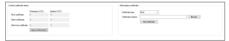
Under the certificates tab, it is possible to upload certificates to your gateway. 3 certificates can be selected in the dropdown menu on the right-hand side. *Root, Client Key* and *Client*. Simply add them one by one and finish the upload by pressing "Apply certificate(s)" on the left-hand side. Note that pressing "Apply Changes" instead of "Apply certificate(s)" will not upload the certificates.
