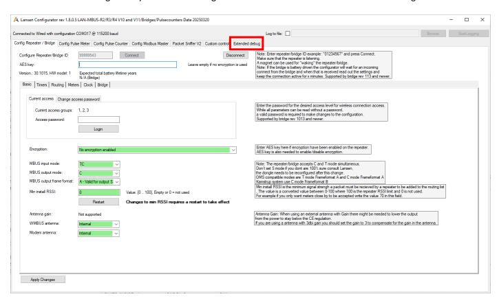
This area of the configurator allows you to see the AT commands to further debug and see what is going on with the gateway if needed, simply select "Enabled" in the top right corner and it will start, granted the MQTT is active on the gateway. Make sure to disable the extended debugger when you are done looking at the AT commands.
