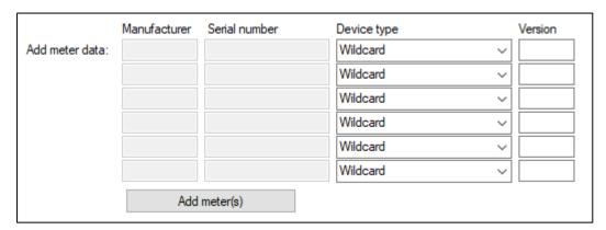
To add a meter to the internal routing list, fill in the manufacturer ID, the serial number, the device type and version, finish by clicking on the button **Add meter(s)**. The meter(s) will then be added to the gateway.
