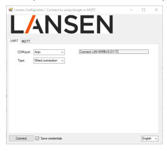
To change the settings to the gateway one must first connect to the gateway. This is done by putting in the serial number which can be found on the poke protection or the front label on the device, then clicking "Connect". Once you have connected to the device you can change all the settings and parameters. The packet sniffer will not be operating when connected through wire.
