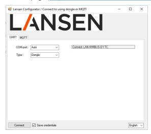
The below window is shown once the connection to the dongle is successful.
