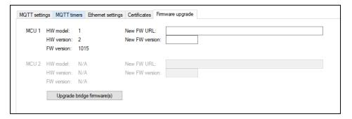
The firmware upgrade tab will allow you to manually update the firmware of the gateway. Simply type in a valid URL to the firmware as well as version number and finish by pressing "Upgrade bridge firmware(s)".
