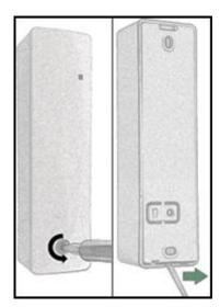
**Note:** If double sided tape is going to be used instead of screws to mount the device, skip to **Step 2b**.
